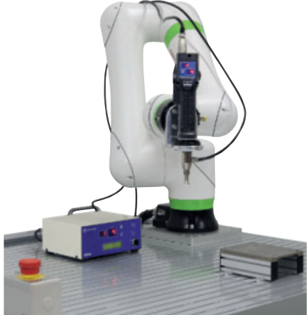
"Delvo" electric screwdriver for automatic screw fastening
